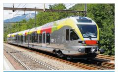
**STA, Italy,** 2013 - 2014 10 FLIRT EMU (15 kV AC/3kV DC)
